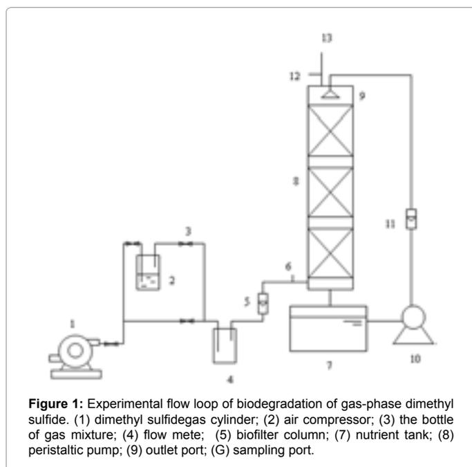
Figure 1: Experimental flow loop of biodegradation of gas-phase dimethyl sulfide. (1) dimethyl sulfide gas cylinder; (2) air compressor; (3) the bottle of gas mixture; (4) flow meter; (5) biofilter column; (7) nutrient tank; (8) peristaltic pump; (9) outlet port; (10) sampling port.
