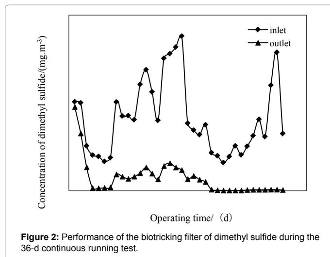
Figure 2: Performance of the biotrickling filter of dimethyl sulfide during the 36-d continuous running test.
