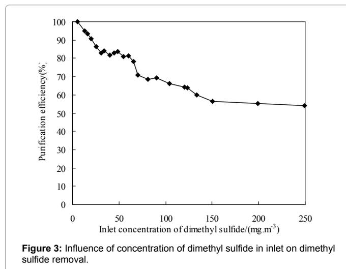
Figure 3: Influence of concentration of dimethyl sulfide in inlet on dimethyl sulfide removal.
