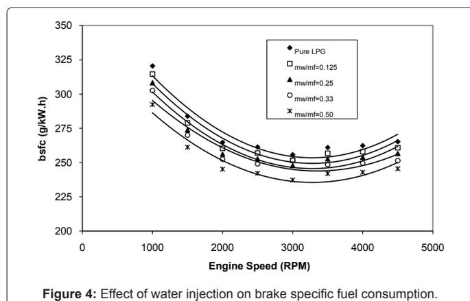
Figure 4: Effect of water injection on brake specific fuel consumption.
