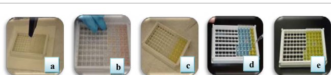
Figure 4: ELISA screening for Malachite Green and Gentian Violet: a) Addition of standards and samples to the ELISA plate, b) Picture depicting the change in color after the addition of 1X Biotin conjugate to the wells, c) Addition of 1X Streptavidin conjugate to the wells, d) Addition of substrate results in formation of blue color, and e) ELISA plate in its last stage where the addition of stop solution develops yellow color and intensity of this color depicts the presence or absence of the Malachite Green and Gentian Violet.
