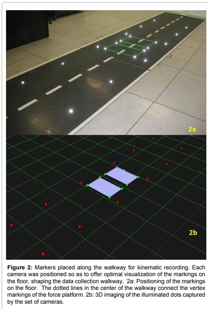
**Figure 2:** Markers placed along the walkway for kinematic recording. Each camera was positioned so as to offer optimal visualization of the markings on the floor, shaping the data collection walkway. 2a: Positioning of the markings on the floor. The dotted lines in the center of the walkway connect the vertex markings of the force platform. 2b: 3D imaging of the illuminated dots captured by the set of cameras.
