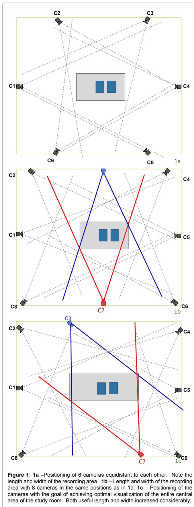
Figure 1: 1a –Positioning of 6 cameras equidistant to each other. Note the length and width of the recording area. 1b – Length and width of the recording area with 8 cameras in the same positions as in 1a. 1c – Positioning of the cameras with the goal of achieving optimal visualization of the entire central area of the study room. Both useful length and width increased considerably.
