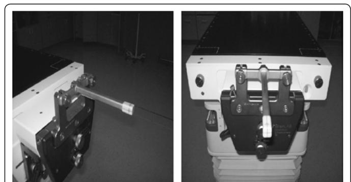
Figure 1: The setup from two different views for a Winston-Lutz test with the simulated target ball at the isocenter.
