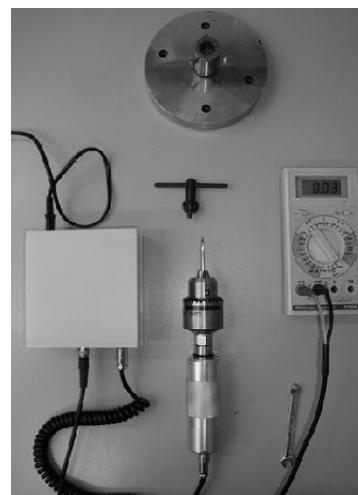
**Figure 3:** Torsionmeter device and experimental set-up tools used for mechanical debonding test.
