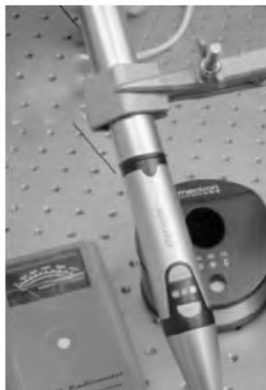
Figure 2: Experimental LED light curing unit used for sample preparation and custom made support for optical tip positioning.
