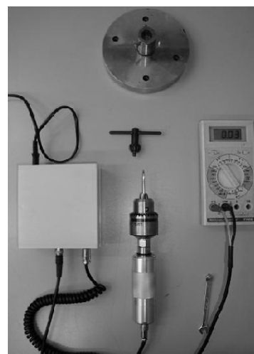
Figure 3: Torsionmeter device and experimental set-up tools used for mechanical debonding test.
