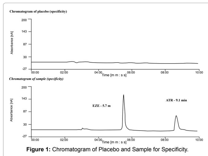
Figure 1: Chromatogram of Placebo and Sample for Specificity.
