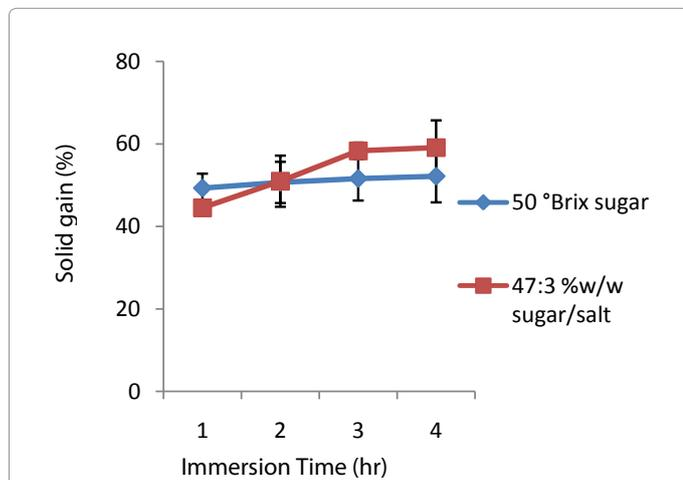
Figure 1a: Solid gain during osmotic dehydration of pineapple slices in sugar, and sugar/salt solutions.
