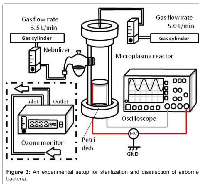
Figure 3: An experimental setup for sterilization and disinfection of airborne bacteria.
