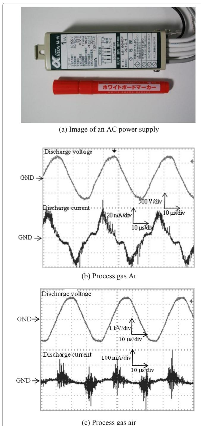
**Figure 5:** Image of a small AC power supply (a), typical waveform of microplasma with AC neon transformer for both Ar (b) and air microplasma (c).
