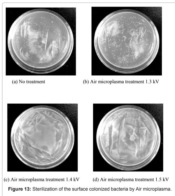
Figure 13: Sterilization of the surface colonized bacteria by Air microplasma.
