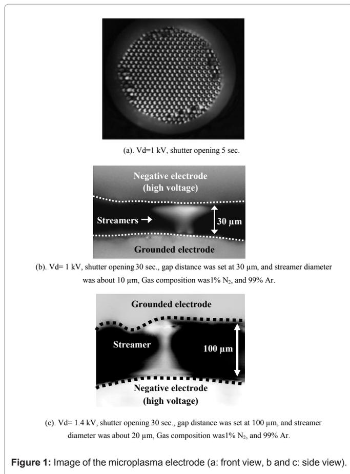
Figure 1: Image of the microplasma electrode (a: front view, b and c: side view).
