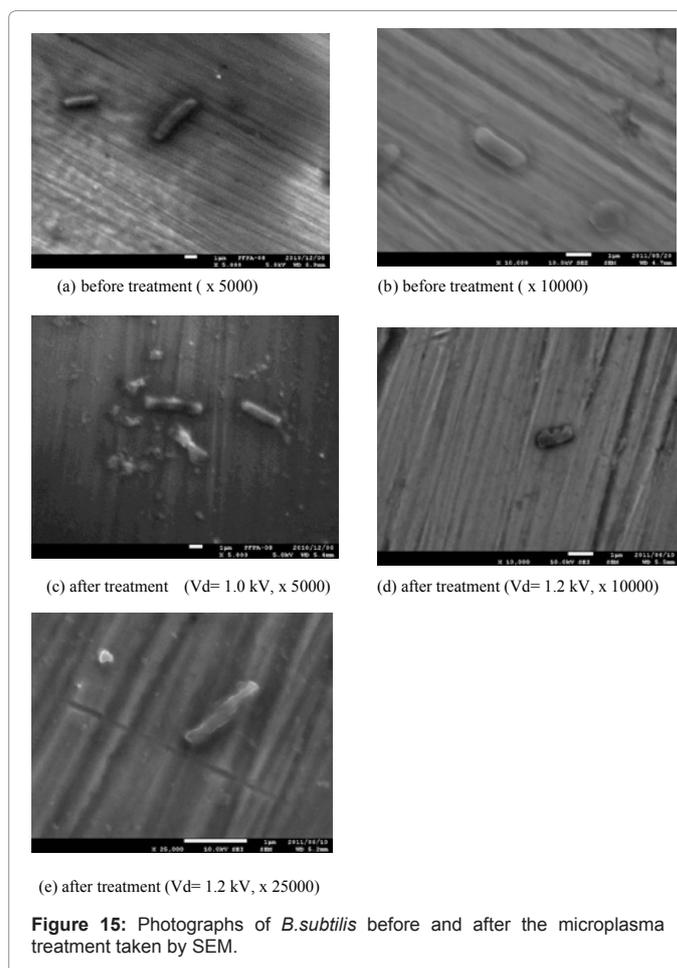
Figure 15: Photographs of *B. subtilis* before and after the microplasma treatment taken by SEM.
