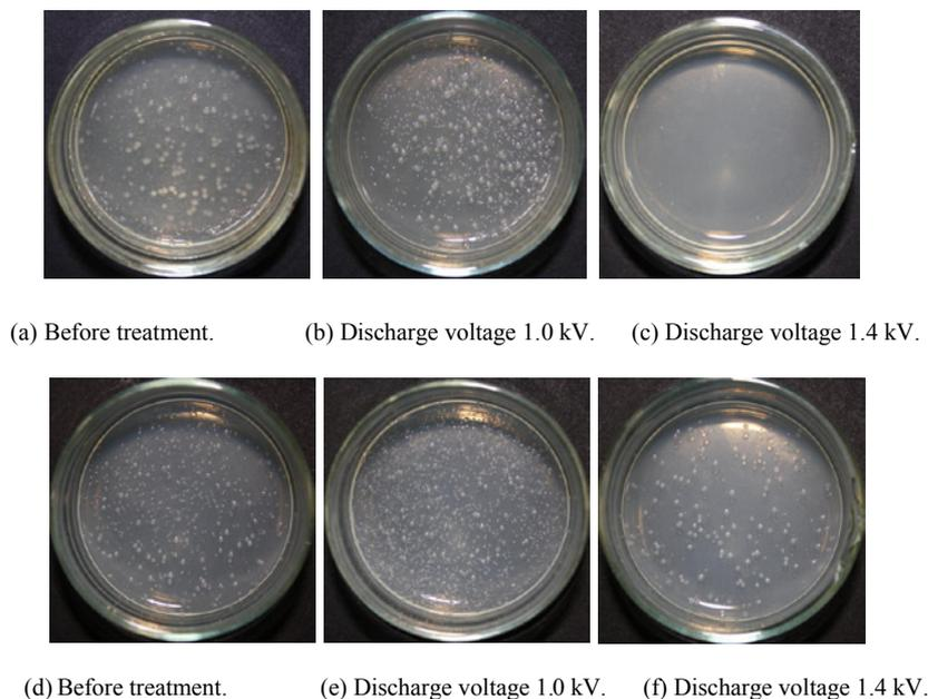
**Figure 8:** Images of the airborne bacteria (*E. coli* JCM20135) colonies before and after the air plasma treatment ((a)-(c)) and that for the nitrogen plasma treatment ((d)-(f)).
