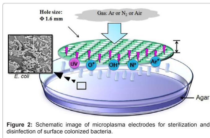
Figure 2: Schematic image of microplasma electrodes for sterilization and disinfection of surface colonized bacteria.
