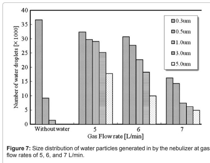
Figure 7: Size distribution of water particles generated in by the nebulizer at gas flow rates of 5, 6, and 7 L/min.
