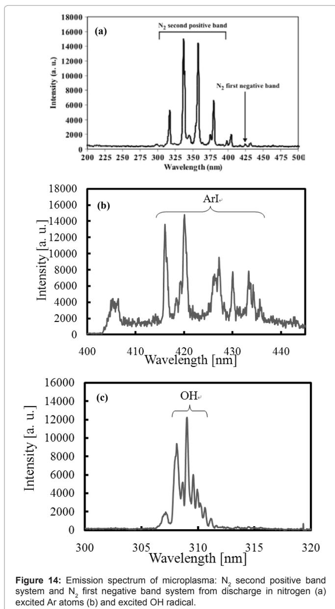
Figure 14: Emission spectrum of microplasma: N<sub>2</sub> second positive band system and N<sub>2</sub> first negative band system from discharge in nitrogen (a) excited Ar atoms (b) and excited OH radical.
