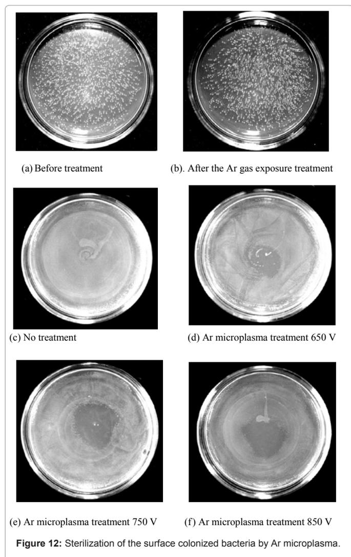
Figure 12: Sterilization of the surface colonized bacteria by Ar microplasma.
