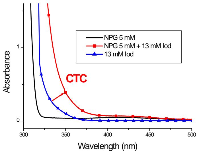
**Figure S1:** UV-vis absorption spectra in DCM of i) 5 mM NPG ; ii) 5 mM NPG+ 13 mM Iod and iii) 13 mM Iod showing the formation of a [NPG-Iod]CTC
