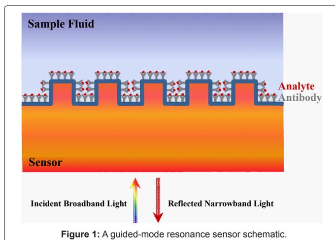
Figure 1: A guided-mode resonance sensor schematic.
