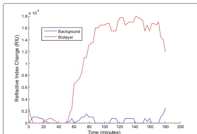
**Figure 4:** Refractive indices of the biolayer and background determined by backfitting the results in figure 3 to a numerical model. The background refractive index remains constant during this particular reaction.
