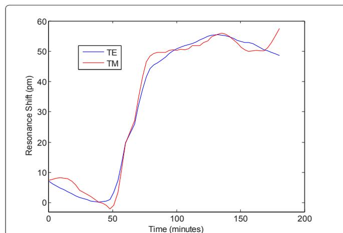
**Figure 3:** Measured biolayer temporal dynamics for a 68 nM solution of calreticulin binding to anti-calreticulin in a PBS solution. We record both polarization states for the lowest waveguide modes.
