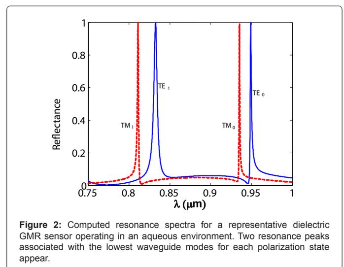
Figure 2: Computed resonance spectra for a representative dielectric GMR sensor operating in an aqueous environment. Two resonance peaks associated with the lowest waveguide modes for each polarization state appear.
