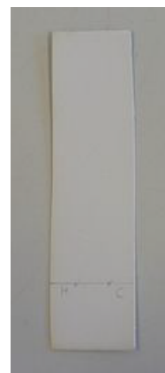
Figure 2: A TLC plate with silica gel coating which is stationary phase.
